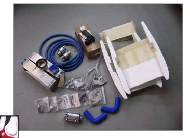
Supermarine Aircraft under wing radiators are designed to produce thrust, increase cruse speed and look like the original plane. The cowls can be use as dummies for air cooled engine.
